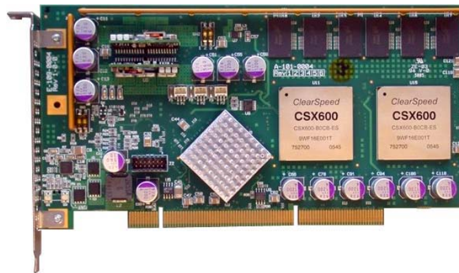
Figure 1 - ClearSpeed's Advance™ X620 accelerator
